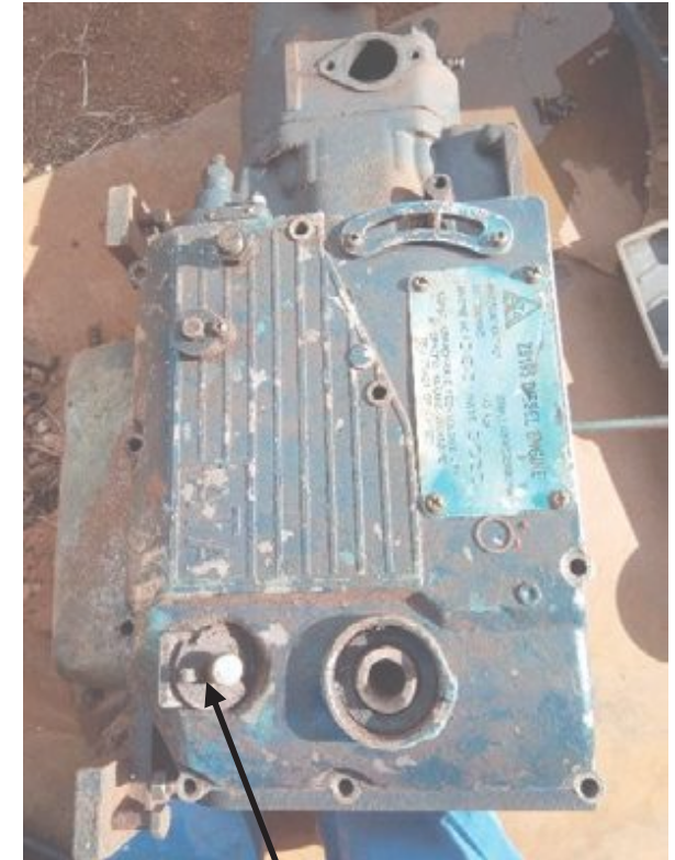
Gearbox dipstick in position after installation
