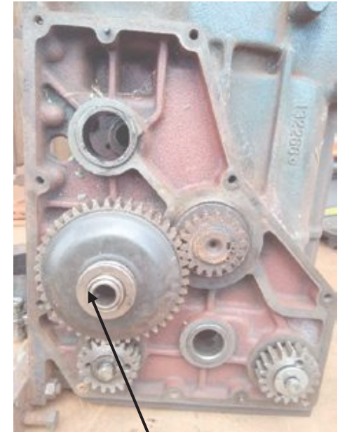
Timing gear in position after installation
