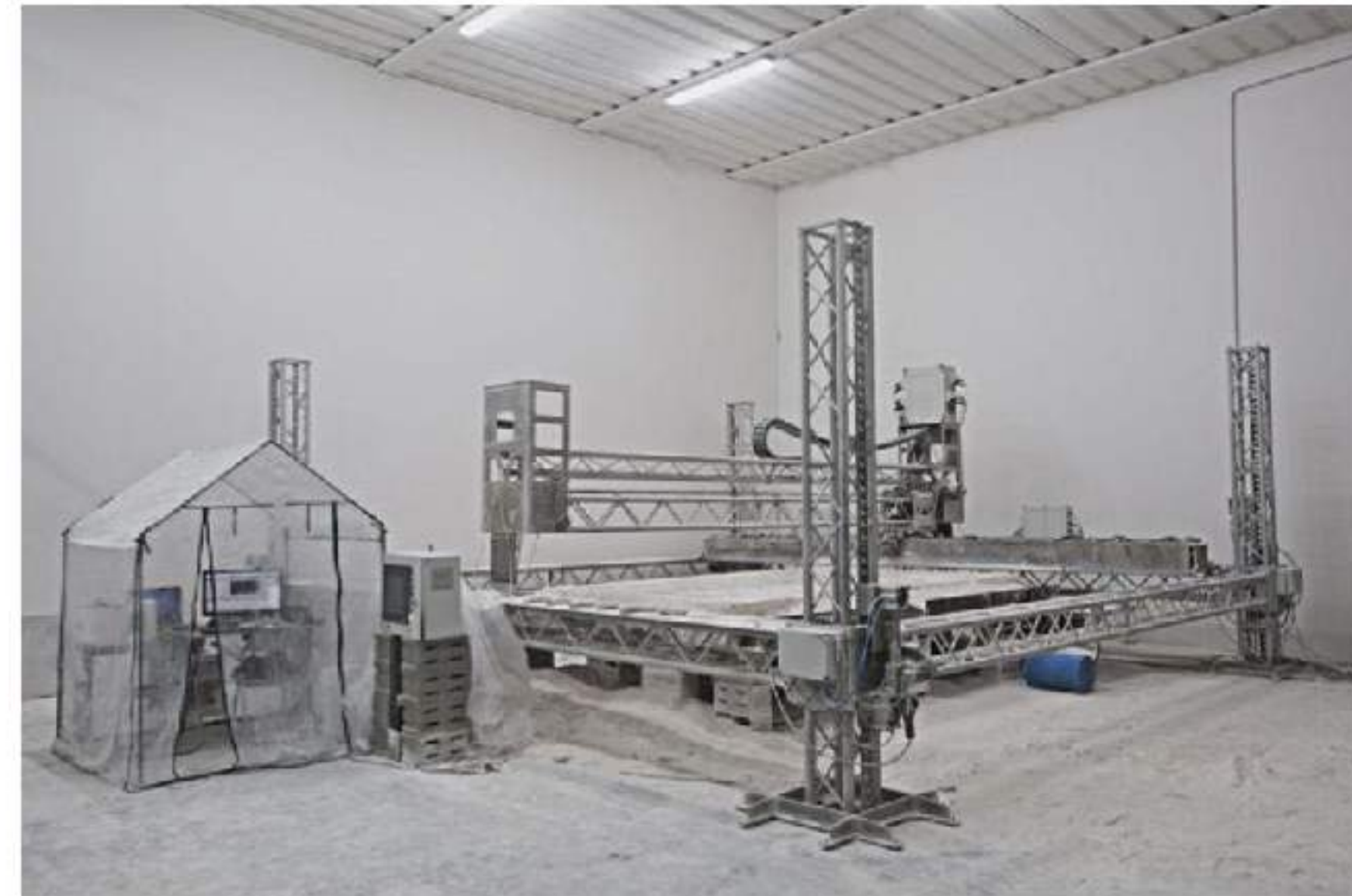
3D Shape printer in process of producing an artificial reef
