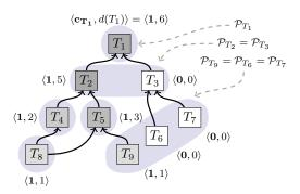
Fig. 11: Example of  $\langle chit, confidence \rangle$  values. Darker boxes indicate transactions with higher confidence values. At most one transaction in each shaded region will be accepted.
