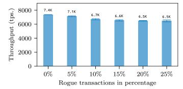
Fig. 18: Throughput vs. ratio of rogue transactions.
