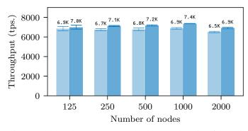
Fig. 13: Throughput vs. network size. Each pair of bars is produced with batch size of 20 and 40, from left to right.
