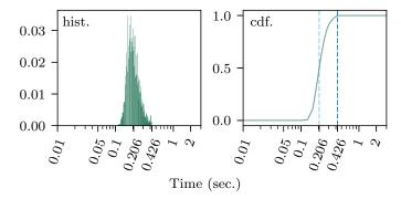
Fig. 15: Transaction latency distribution for n = 2000. The x-axis is the transaction latency in log-scaled seconds, while the y-axis is the portion of transactions that fall into the confirmation time (normalized to 1). Histogram of all transaction latencies for a client is shown on the left with 100 bins, while its CDF is on the right.
