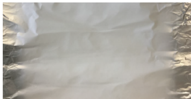
Figure 2. Electrospun PVL membrane on the aluminum foil.
